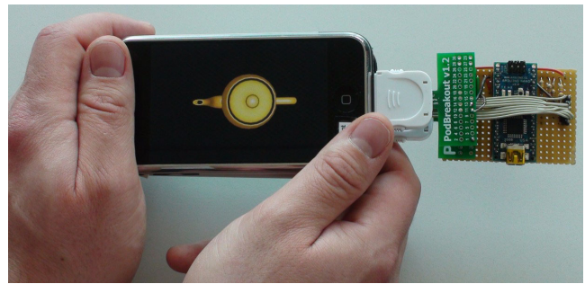
Figure 1. Sandwich prototype for two-sided multitouch sensing with continuous pressure input.
