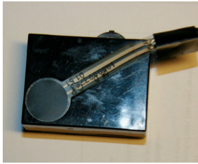
Figure 11. Shake device for vibrotactile feedback with FSR on top.
