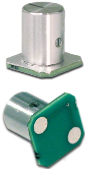
Figure 1 The rotary knob CapWidget is made from aluminum and is attached to a PCB that creates artificial touch points by conveying the user's ground potential to the surface of the touch screen.
