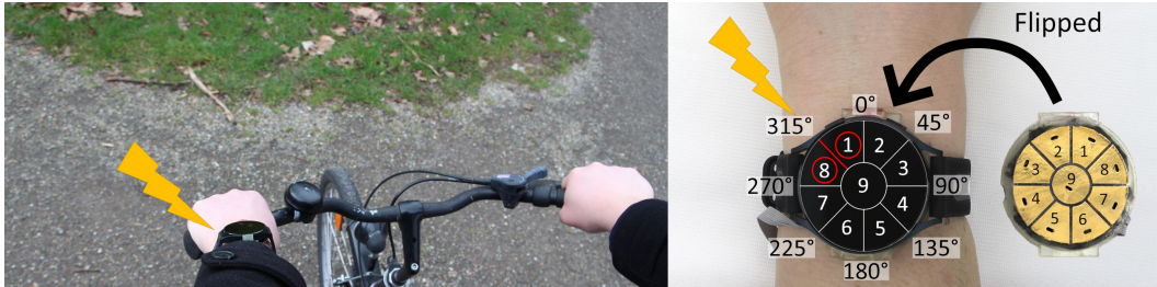
Fig. 1. Left: A user in front of a junction wearing our directional navigation system under the smartwatch. He receives electrotactile feedback that informs him to take the left road. Right: The user feels the electrotactile sensation on the upper left part of the watch (electrodes 1 & 8), which indicates taking the left road. The electrode grid is attached to the back of the smartwatch.
