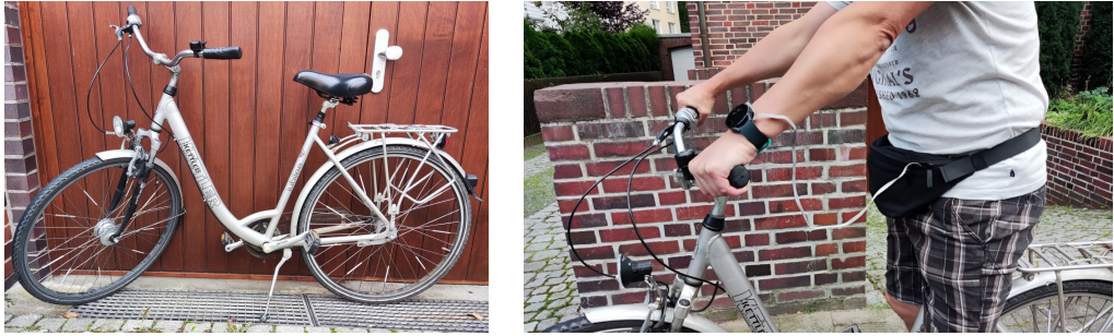
Fig. 7. Left: The bicycle used in the study. Right: A participant on the bicycle wearing the electrode grid under the smartwatch on the left wrist. The Rehamove 3 and other components are located in the waist bag.
