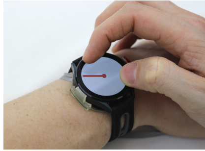
Fig. 4. A participant is rotating the handle on the smartwatch touchscreen with two fingers to match the handle's orientation with the presented electrotactile feedback.
