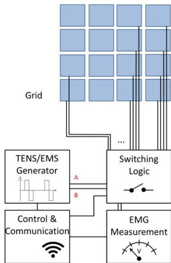
**Figure 2:** Components of the planned electrode grid. The EMS generator produces the stimulation signals, which are directed to different electrode configurations over the switching logic. A control and communication unit synchronizes the components. It controls the stimulation parameters and collects the measurements from the EMG unit.
