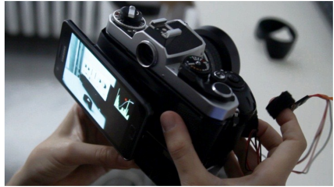
Figure 9. Tickle interface implementation on an Android phone for testing 2-finger camera control on a real SLR form factor.
