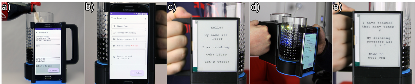
Figure 1: CheersMate features involving public and private wearable displays: (a) ingredient levels and instructions for mixing drinks on the private display, (b) drinking statistics screen on the private display, (c) default screen on the public display welcoming others, (d) two CheersMates clinking, and (e) shared statistics on the public display.
