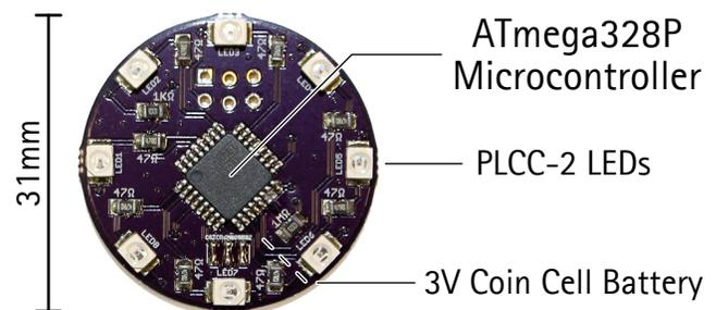
Figure 2. The central part of our prototype is a custom PCB containing 8 LEDs. The LEDs are controlled with a microcontroller and powered from a coin cell battery mounted on the back of the PCB. This board is sized to fit snugly into an empty watch case.
