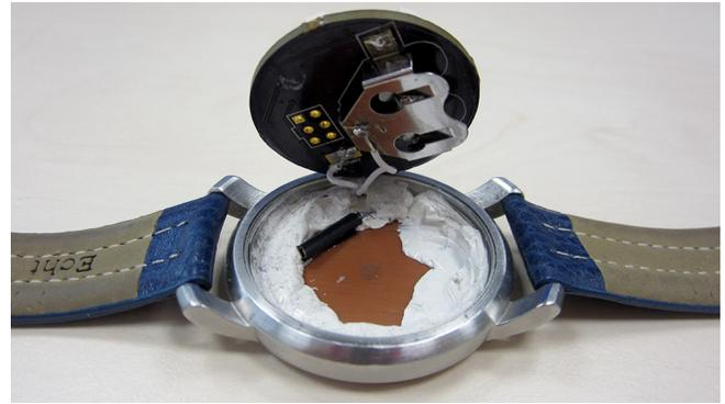
**Figure 5.** The bottom of the PCB holds a coin cell battery with enough power to run the prototype for a day. We sealed the front of the watch to prevent light leakage to the front. The used putty also holds the PCB in place and prevents damage due to free movement inside the case.
