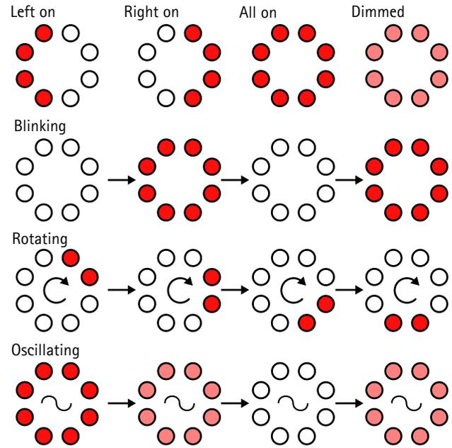
**Figure 8.** The LEDs in our prototype can display seven different patterns. Four of them are static, while the remaining three are animations.
