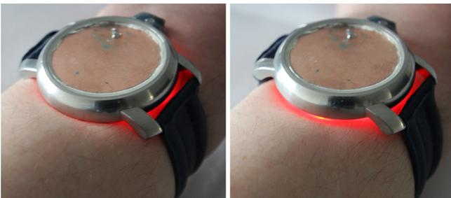
**Figure 4.** When wearing the watch directly on the arm (left) it sits tighter than when using the silicone padding (right). The slight gap due to the silicone also leads to additional light on top of the scattered one.
