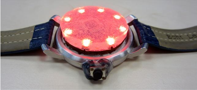
**Figure 3.** We cover the LEDs in a 4 mm thick layer of clear silicone for added comfort. This prevents the hard edges of the LED housings from irritating the skin, while still allowing light to pass through.
