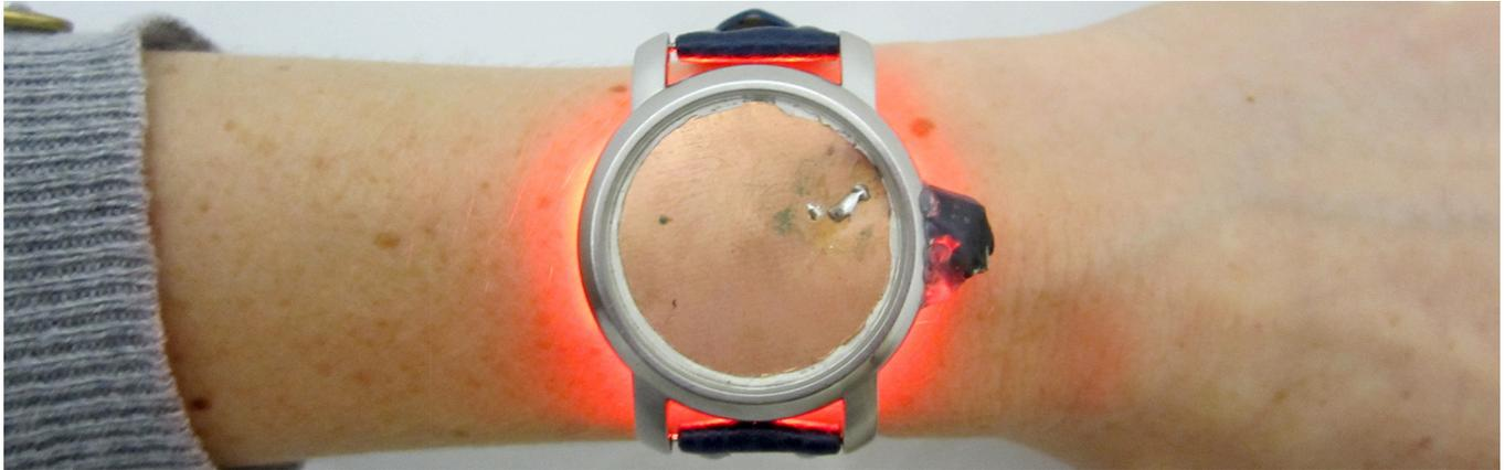
Figure 1. We added LEDs to the bottom of a watch case for use as a notification mechanism. The red light can pass through skin, scatters, and can be observed all around the watch. This enables a more subtle means of feedback—not as disruptive as vibration and more connected to the body than outward-facing illumination. This kind of indirect illumination feedback is still noticeable to users and visible through some clothing.
