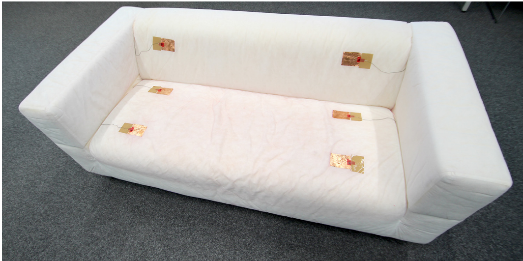
Figure 1: We attached six electrodes on the couch. In use, those electrodes are hidden underneath the couch cover.
