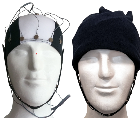
Figure 1: HapticHead prototype with 24 actuators around the head and high-density areas on the forehead and chin. Left: Raw prototype; right: integrated into a beanie. Built after the concept of Kaul et al. [6].
