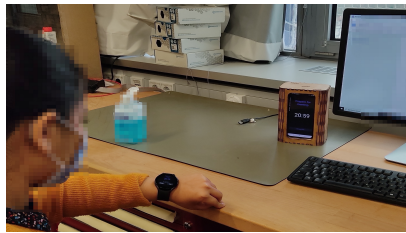
(a) Desk: UWA assisting the user to focus on the task. The S-CA is placed on the desk (casing left of the monitor) and the W-CA is attached to the user's wrist.
